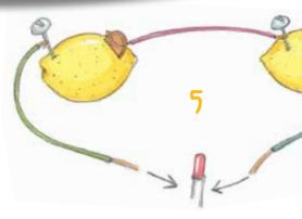
**5** Now take the other lemon and stick the corresponding coin and screw into it. Connect the end of the wire leaving the first screw to the coin in the second lemon and the coin in the first lemon to the screw in the second one. Cut this last wire in half and strip the ends as shown in the drawing: You're going to connect it to an LED.
