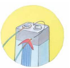
**4** Connect the two ends of the cable to the poles of the battery (the two little bumps at the top of the battery).
